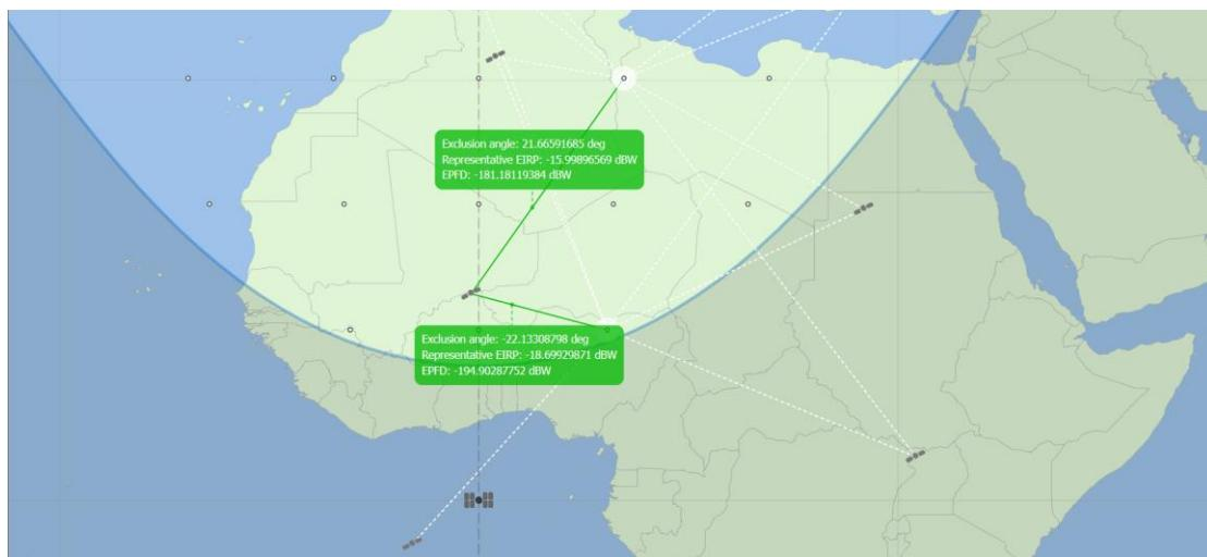
**Figure 18: Showing links between non-GSO satellites and Earth stations**
